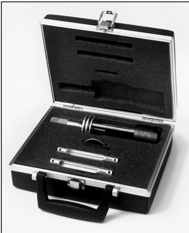
The CMSS 601-1 is supplied as a portable kit complete with standard target disc, an Allen wrench and two adapters to accommodate both CMSS 65 and CMSS 68 Eddy Probes.
