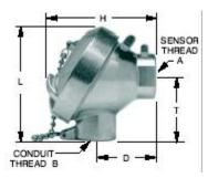
Cast Aluminum Head Silicone Gasket IP 55 Type 3 and 4 3.5 (89) H 3.5 (89) L 2.0 (51) D 1.75 (44) T A = 3/4" NPT B = 1/2" NPT
