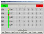
Password protected Setup pages are provided for all monitored parameters and include Tag Name, Status, Full Scale Range, Enable/ Disable, Current Value and 4 Alarm Set Point Values (2 Low, 2 High). Global Alarms at the top of the Screen alert the user to any alarms during setup changes. Multiple pages may be used for high channel count systems.
