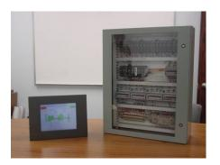
Making use of the world's most popular HMI software (Human Machine Interface), Wonderware Intouch, STI's CMCP-HMI System provides a complete Monitoring System when communicating via digital link to STI's distributed Field IO and Transmitter Based Sensors. It can be used on a single machine or dozens of machines. Each CMCP-HMI is provided with the following basic screens: Machine Mimic, Channel Setup, Alarm List, Historical Alarm List, Real Time Trends and Historical Trend.
